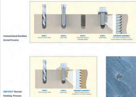
A comparison of the installation processes of a metric fastener and a thread-forming fastener
