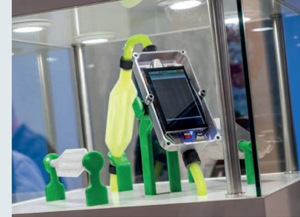
*Aluminium casing for cooling power electronics*
