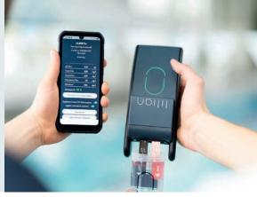
Mobile analysis system for determining water properties and quality
