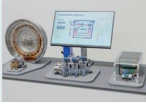
From left to right: a highly integrated valve block, electric motor cooling and battery temperature control
