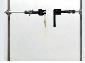
Right: the TIGITAL 3D-Set PPP material; left: a thermoplastic material after a fire test
