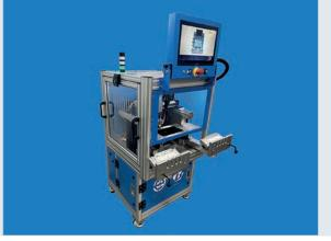
A processing robot for the production of cable splices
