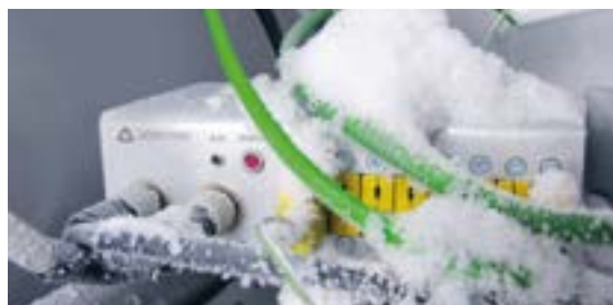
Frozen EPAD Modules - still operating at -40 °C
